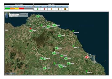
User tracks can also be downloaded in KML format for detailed historical data analysis. The KML log file contains all user positions and the corresponding quality status data for a given connection. Service operators can use this information to monitor service quality and troubleshoot user performance issues.
